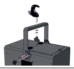
2 Mount the twenty clamp on a truss and secure with a certified safety cable.
