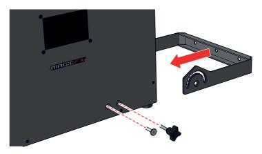
3 Place the MAGICFX® CLUBBLOWER under an angle by rotating the bracket to the bottom side of the machine and tighten the star knobs on both sides.
