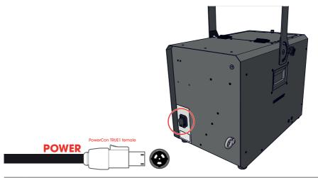
3 Connect the other end of the powerCON TRUE1 cable to the controller or power switch.
