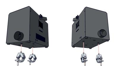
Mount the DOUGHTY® half coupler clamps on a truss and secure with a certified safety cable.
